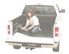
With ribbed side up, lift the mat into the truck bed and tuck it into the channel in the rails. It is generally easiest to tuck one side; then fit the other side. Make sure it is pulled as far forward as possible for best fit. The mat will "settle" into the best fit position over the first hundred miles or so of driving.
