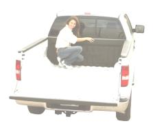
While temperature does not affect your DualLiner, it is easiest to install when the bedliner is above 50 degrees Fahrenheit. If working in colder temperatures, it is helpful to warm the bedliner indoors prior to installation. The mat may take a "set" while rolled. If possible, unroll and let it "relax" in the sun for a little while to make it easier to work with. If installing in cold weather, the mat may take several weeks to fully relax.
